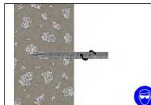
8. Any excess resin should be expelled from the hole evenly around the steel element showing that the hole is full. This excess resin should be removed from around the mouth of the hole before it sets.
