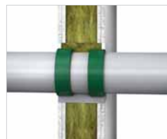
Penetration through flexible and rigid walls ≥ 100 mm.
