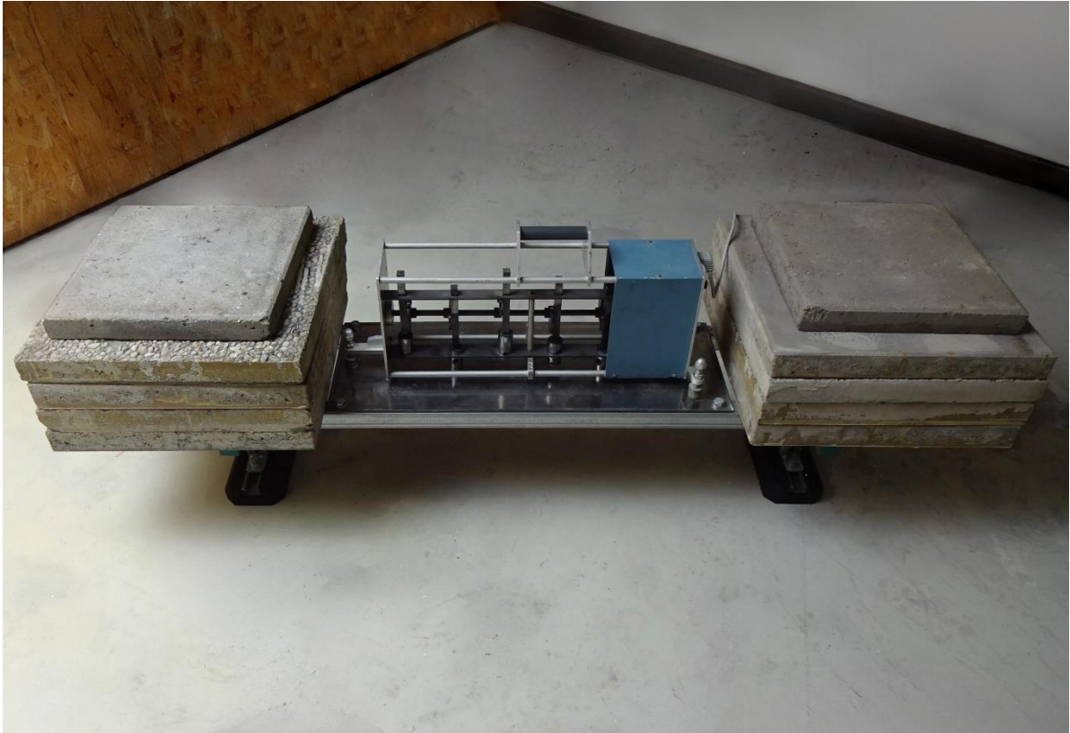
Photo 9: Type A-low, Length = 250 mm, 150 kg weight per foot
