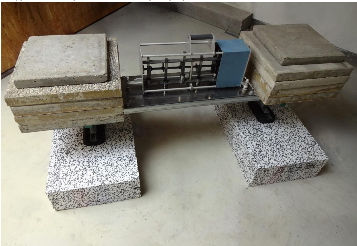
Photo 10: Type A-low, Length = 250 mm, 150 kg weight per foot, with additional EPS-insulation
